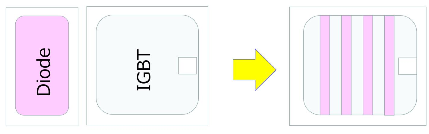
(2)Shorten the interval between IGBT/Diode Material reduction/Number of chip reduction Reduction of assembly cost by reducing connection
