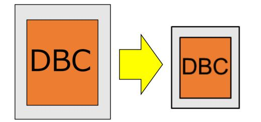
(3) Increased heat dissipation path and area Reduced thermal resistance, Chip downsizing IGBT + Diode **RC-IGBT**
